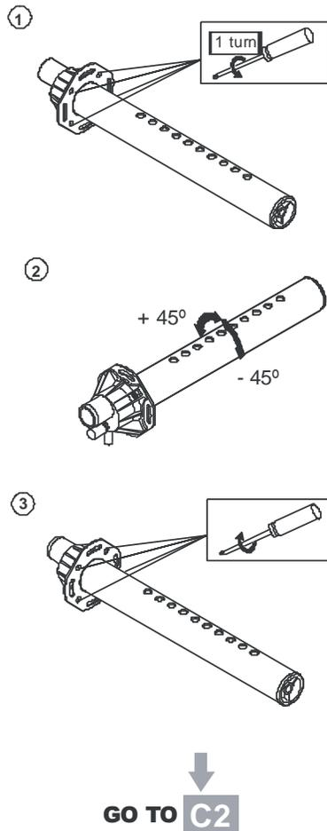
**Figure 6: Vertical Airflow**
